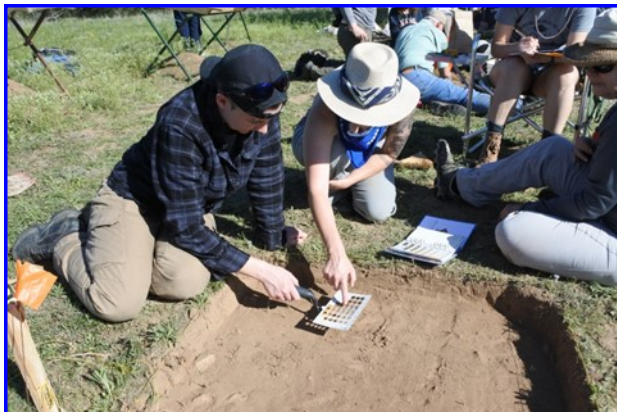
Determining Soil Color using a Munsell Soil Color Chart
